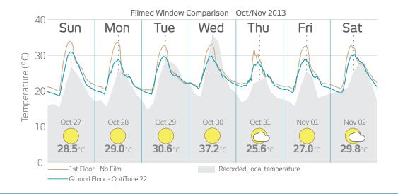
Temperature logging devices installed behind the installed film at ground level, and directly above on the first floor behind unfilmed glass revealed how effective OptiTune 22 is in reducing solar heat gain and thereby lowering the interior room temperature.
